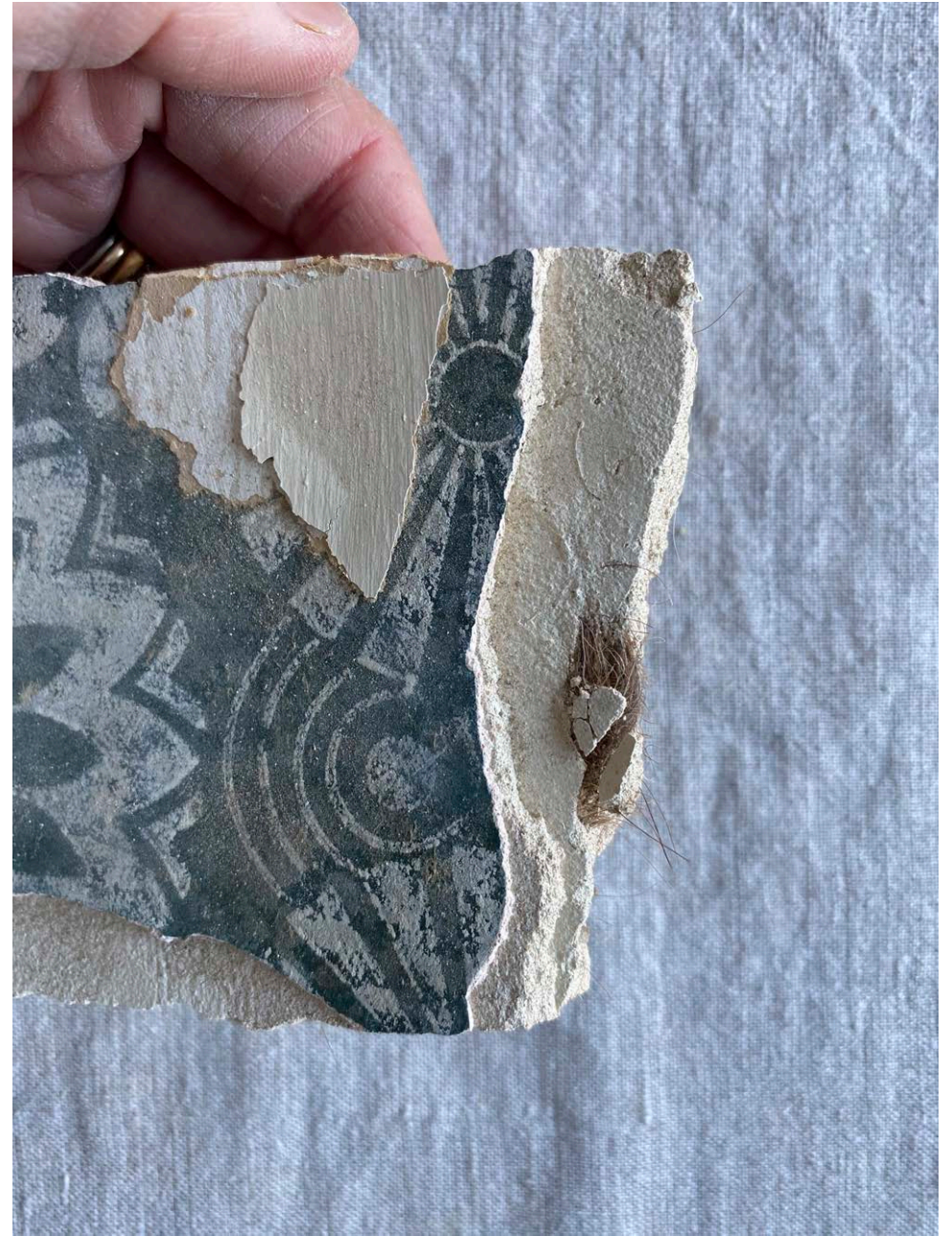
Edge, with tuft of animal hair in the lime plaster
