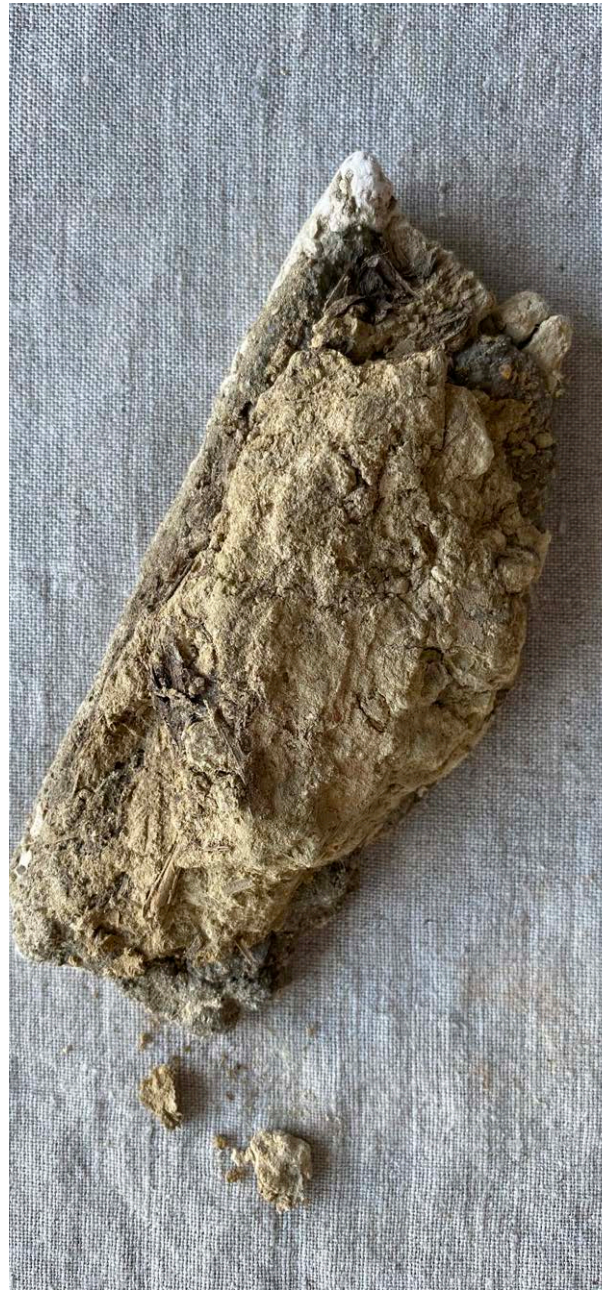
Chunk of plaster with animal hair and straw [from loft?]
