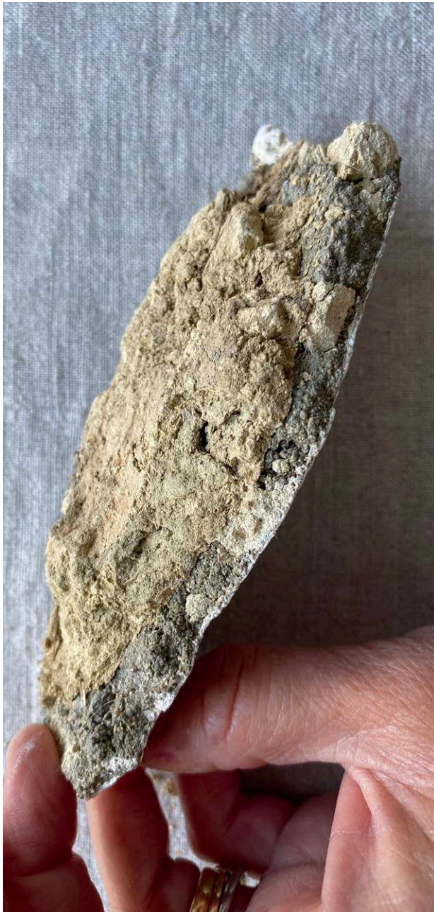
Chunk of plaster with animal hair and straw [from loft?]
